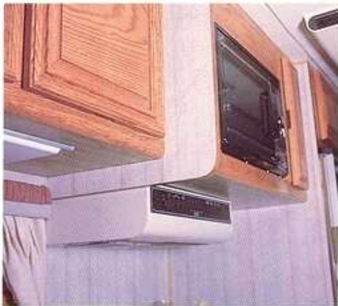
Range Hood w/Monitor Panel.
